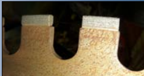
Partially worn blades - diamonds fully exposed
